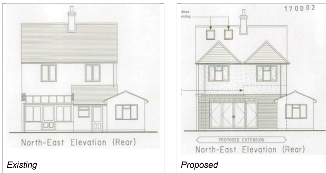
Figure 1 – Existing and Proposed rear elevations
