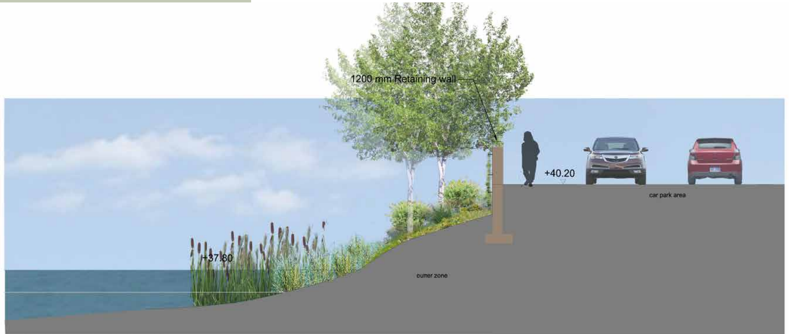
Typical section indicating retaining wall to lake edge
