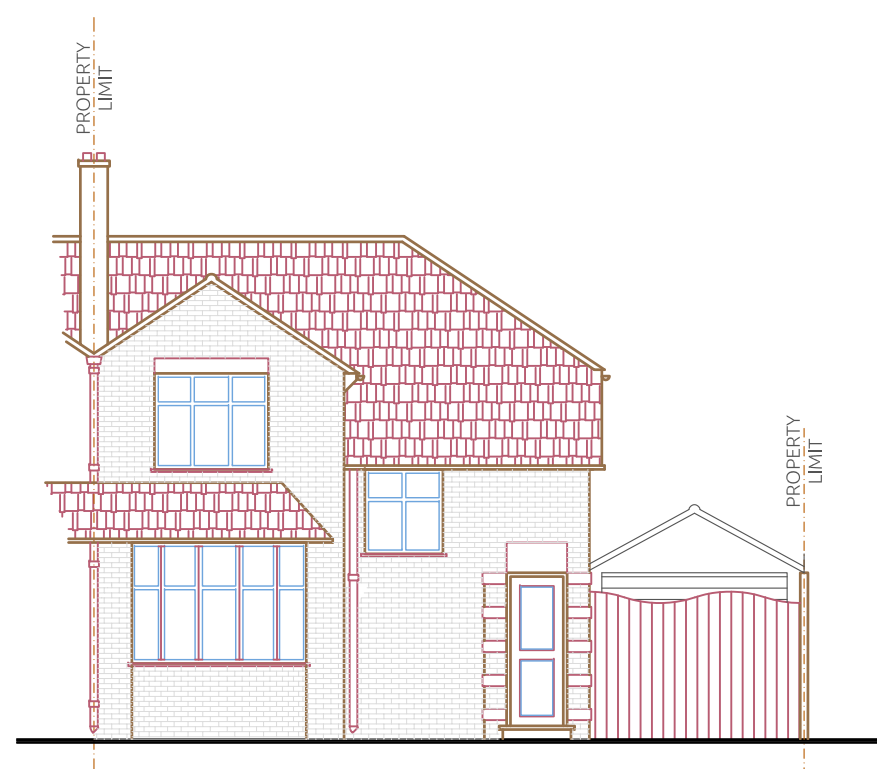
EXISTING Front Elevation
