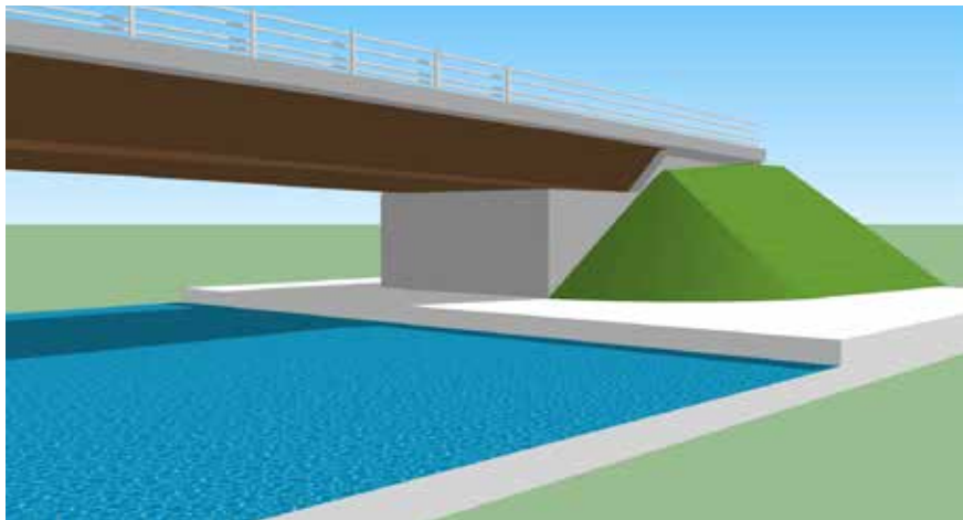
Figure 51. Retaining wall with girder extended over the abutment.
