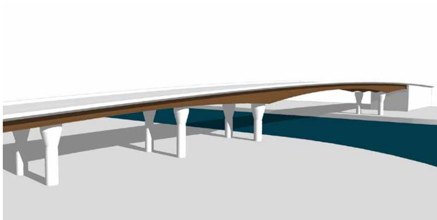
Tapering depth steel girder with retained embankment of west side.
