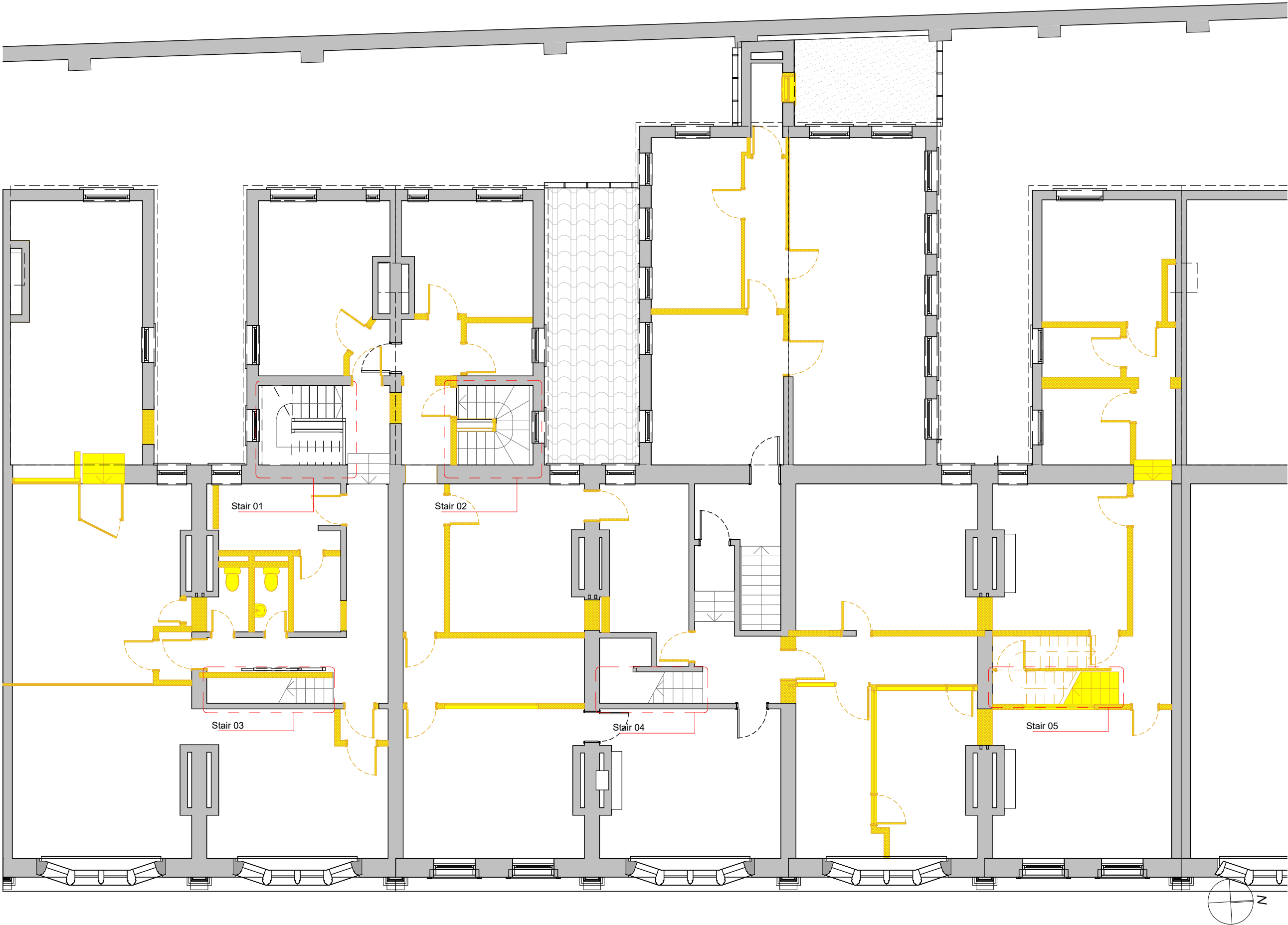
2. First Floor Demolition Plan Scale: 1:100
