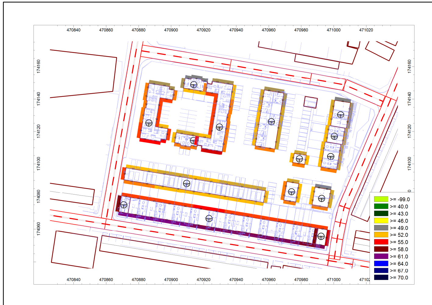
Figure 17: Day L_{Aeq} Building Evaluation (Rail Sources)
