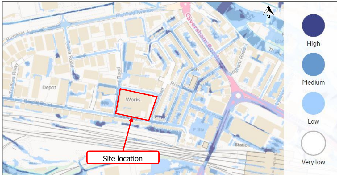
Figure 3: EA Surface water map – Extent of flooding
