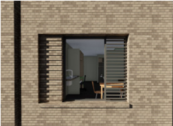
Proposed projecting brick - alternate courses and window louvre vent detail (indicative image)
