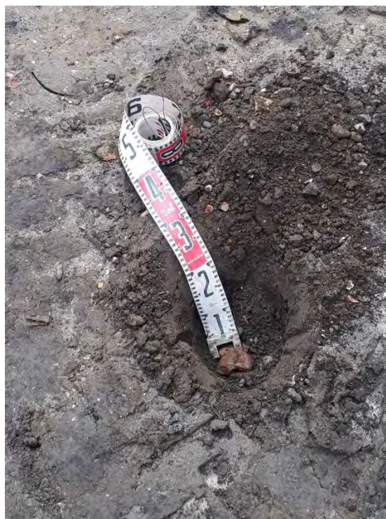
Plate 11: Hand dug pit HD05 undertaken in Plot 3, confirming 300mm of capping.
