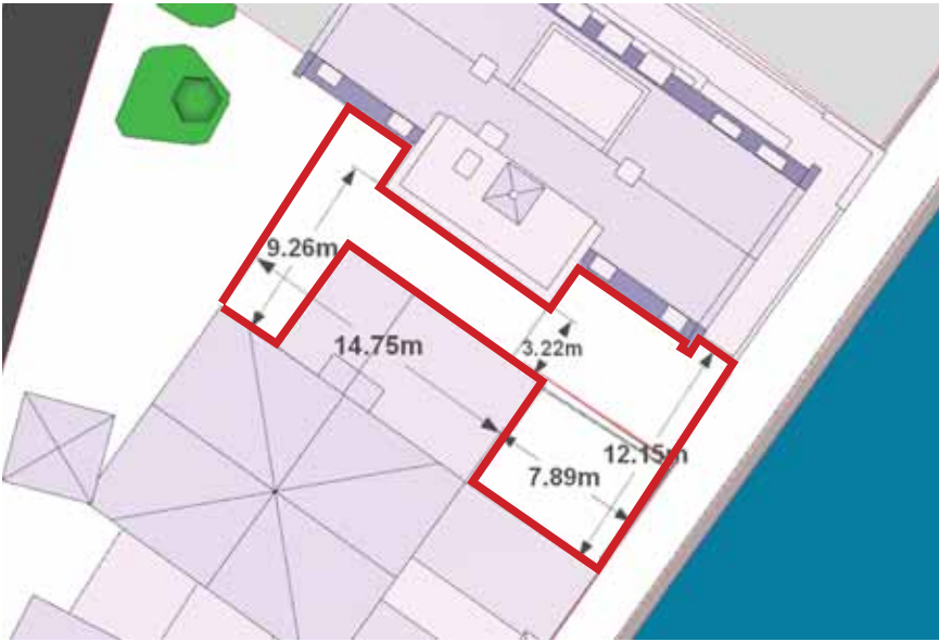
Width of courtyard at ground level: 3.22m
