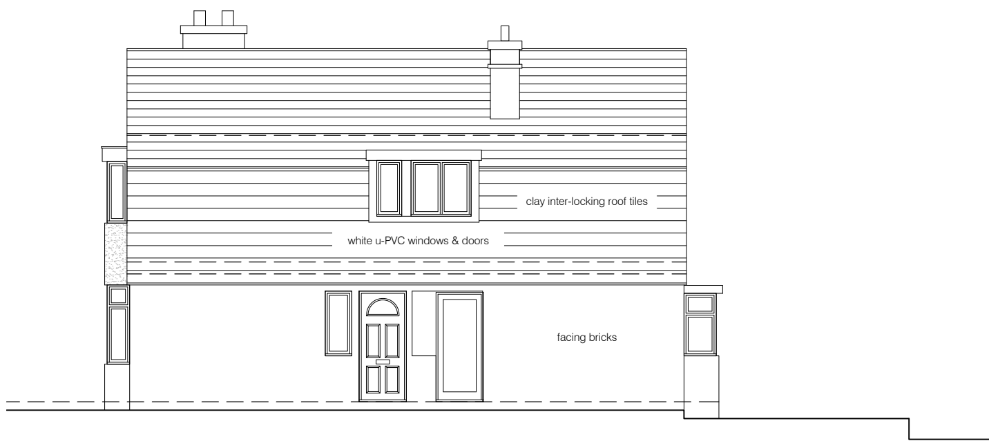
Existing - Side Elevation 1 : 100
