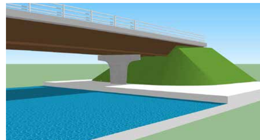
Figure 60. Retaining wall with column and embankment
