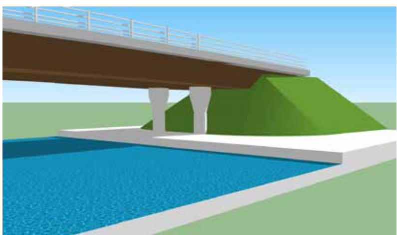
Figure 56. Open abutment with earth embankment
