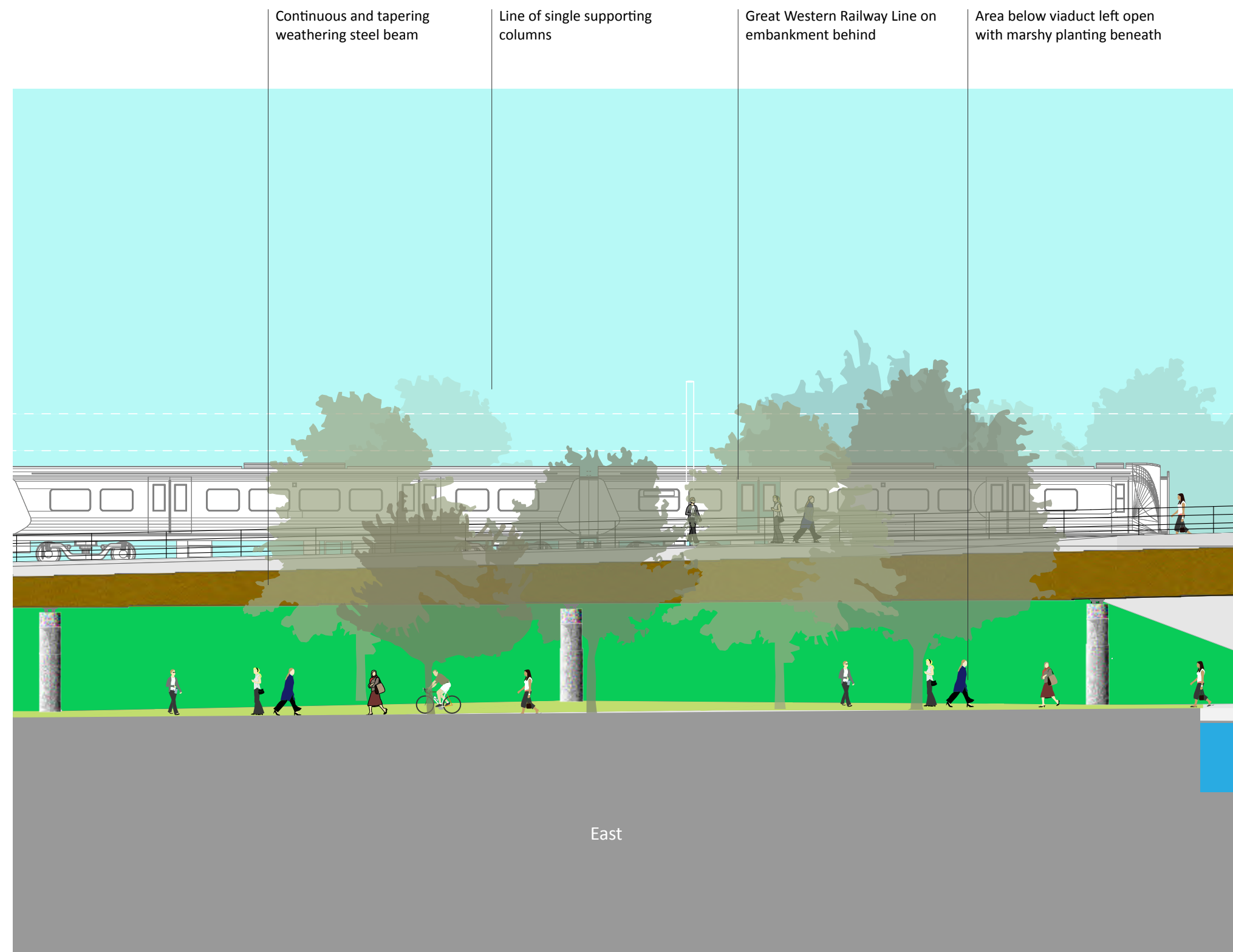
Figure 45. Selected bridge form (tree planting shown indicatively)
