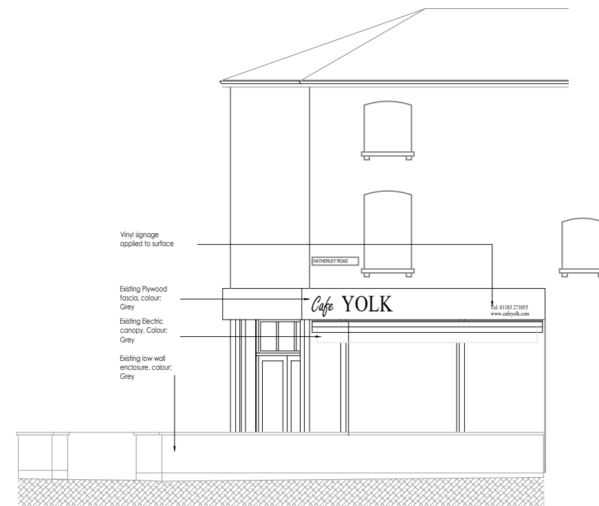
3 West Elevation Hatherley Road SCALE 1:100
