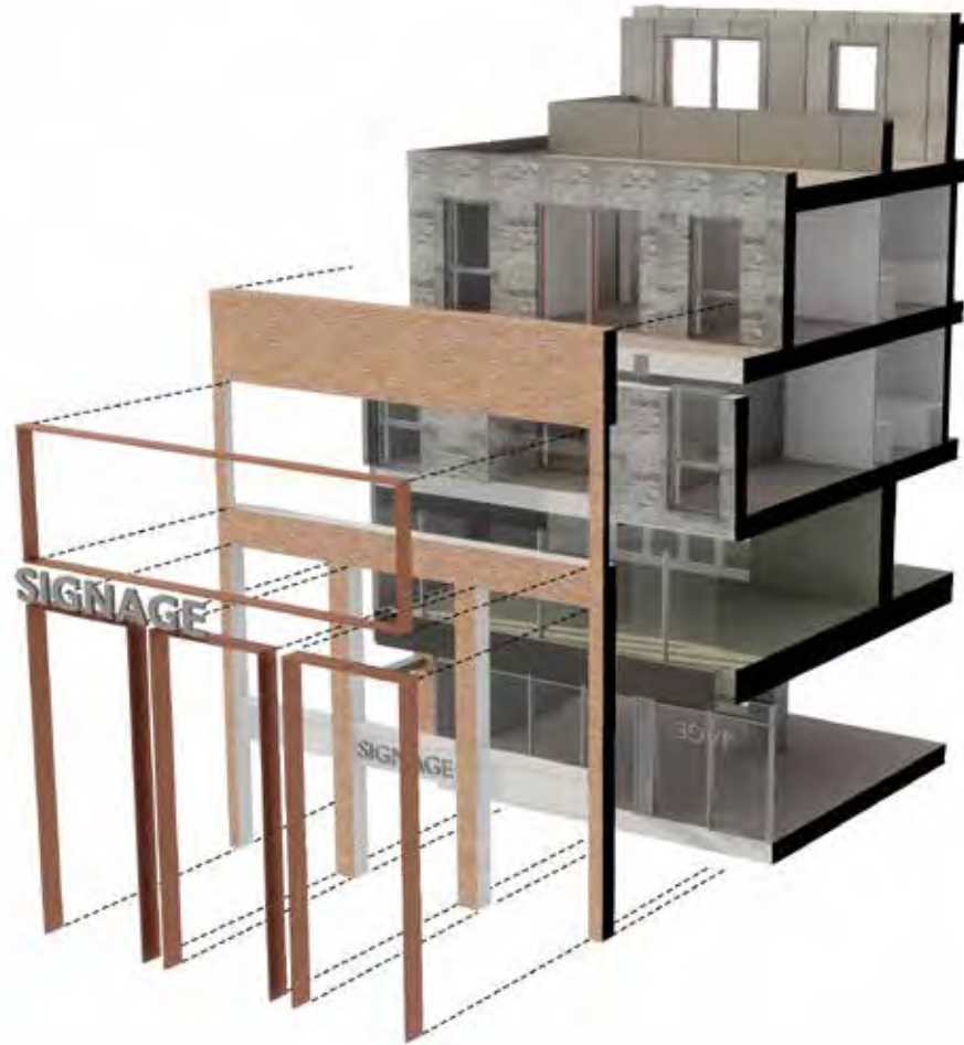
fig. 50 Exploded view of facade construction
