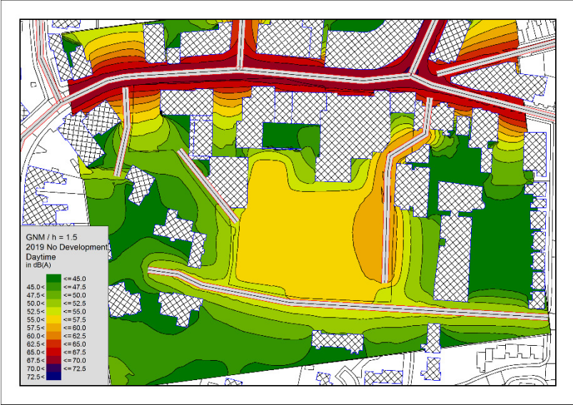
Figure 7 - Grid Noise Map showing noise propagation for 2019 No Development scenario
