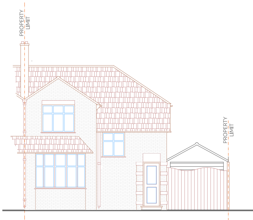
Existing Front Elevation
