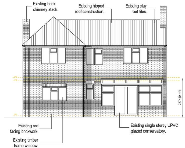
Figure 13: Existing Rear Elevation (Materiality)
