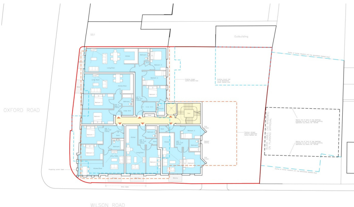
Proposed 1 st Floor Plan (2 nd Floor is identical) showing living rooms facing the street and bedrooms to the rear
