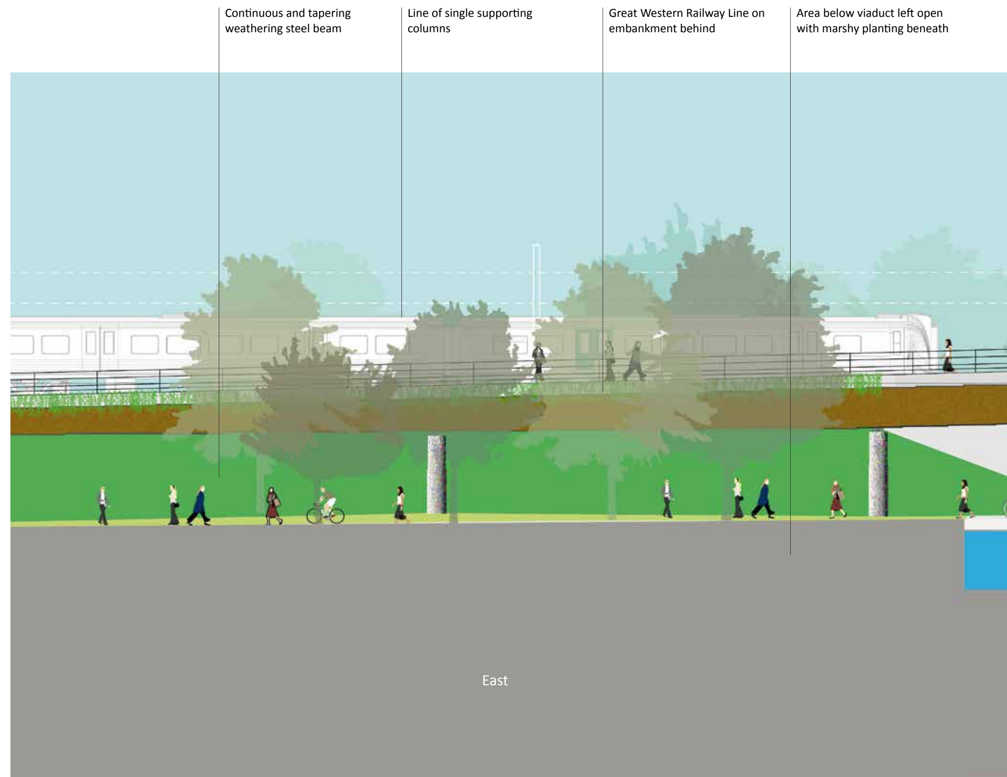
Figure 64. Selected bridge form (tree planting shown indicatively)
