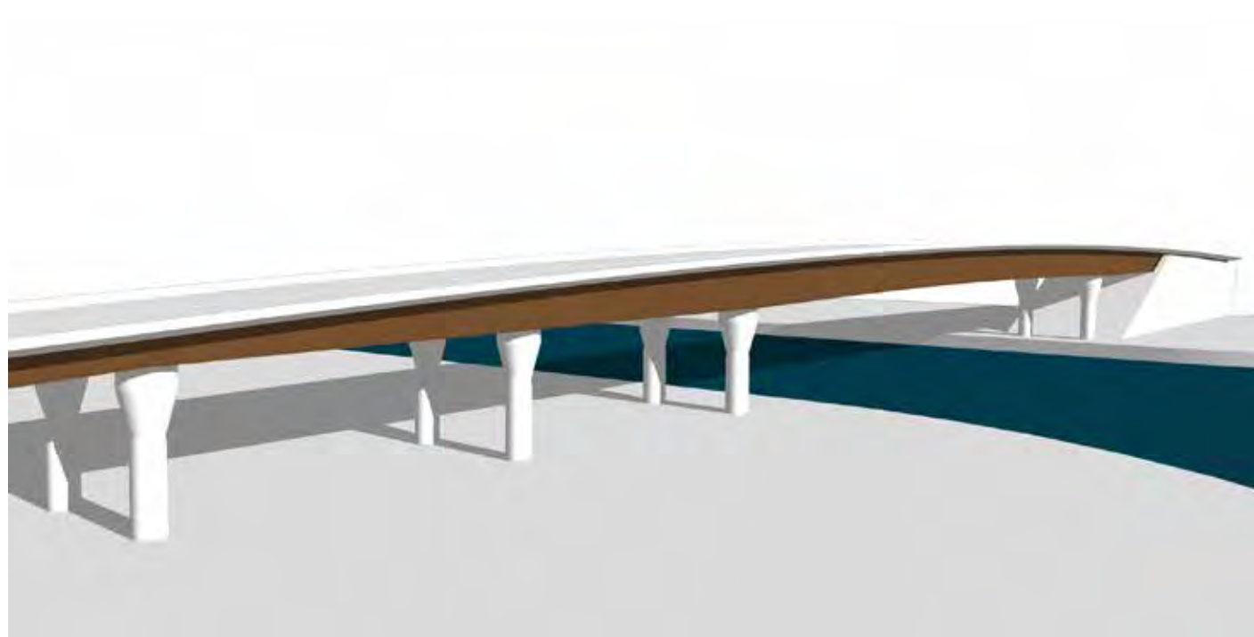
Deep, gently cambered girder to main river span tapering to the east and west with part enclosed abutment to the west.
