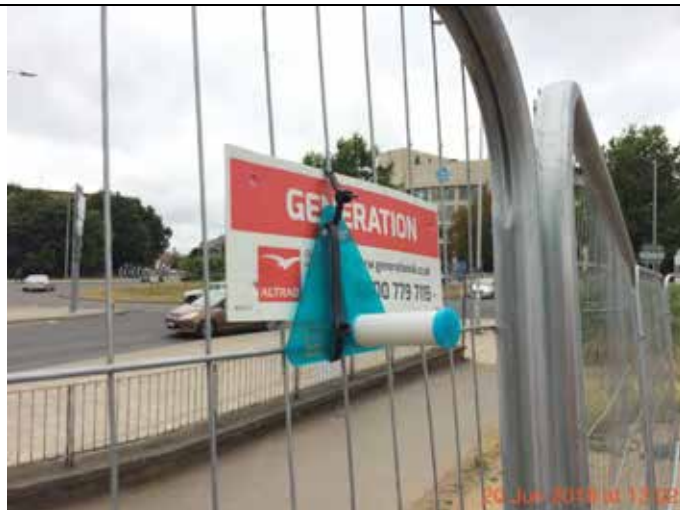
Photograph 11 – VOC monitoring points set up along the four site boundaries.
