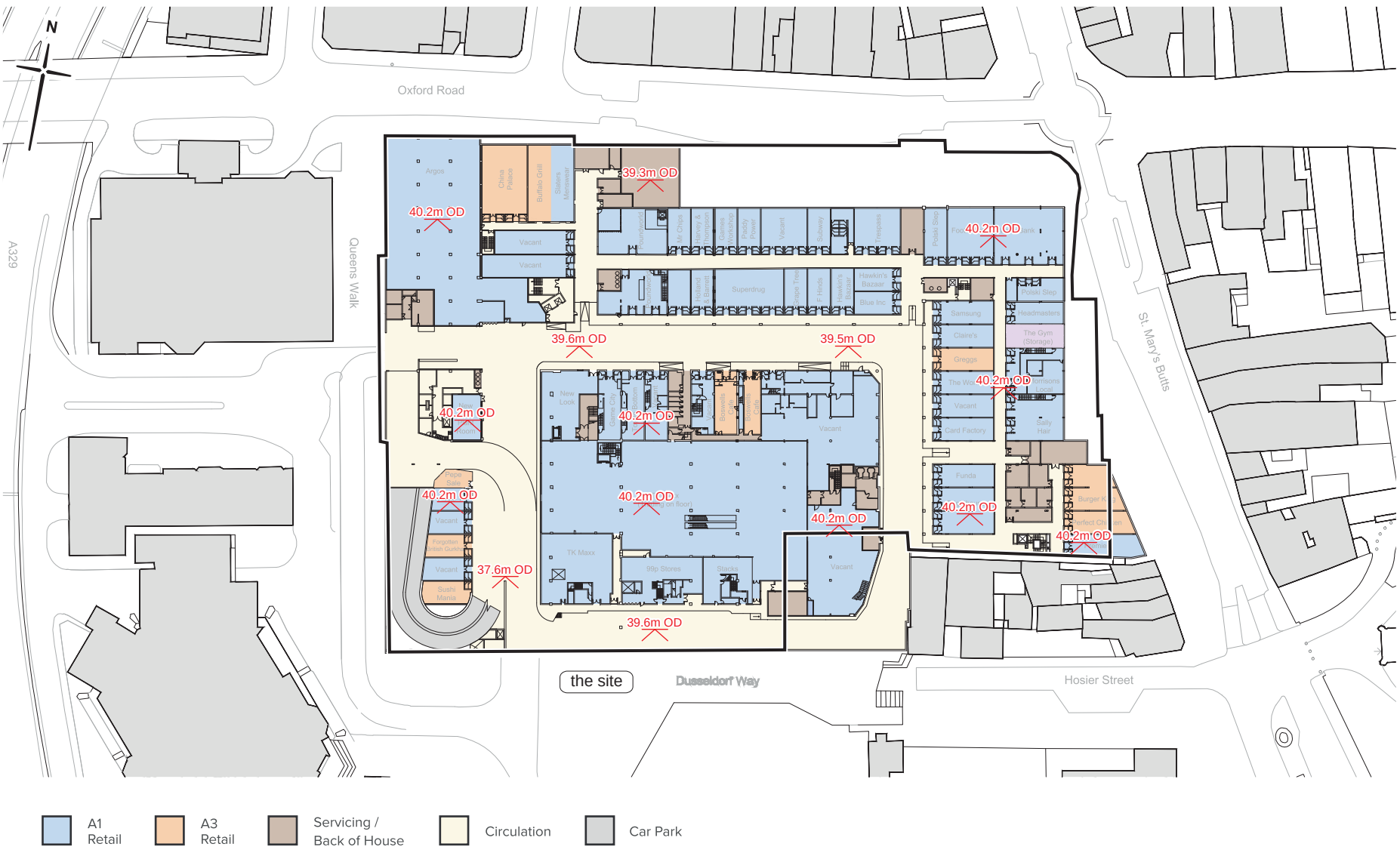
Fig 4b Existing basement plan showing levels taken from site survey (Corstorphine and Wright Architects, October 2016; Warner Surveys, Job No.S715/0357, May 2017)
