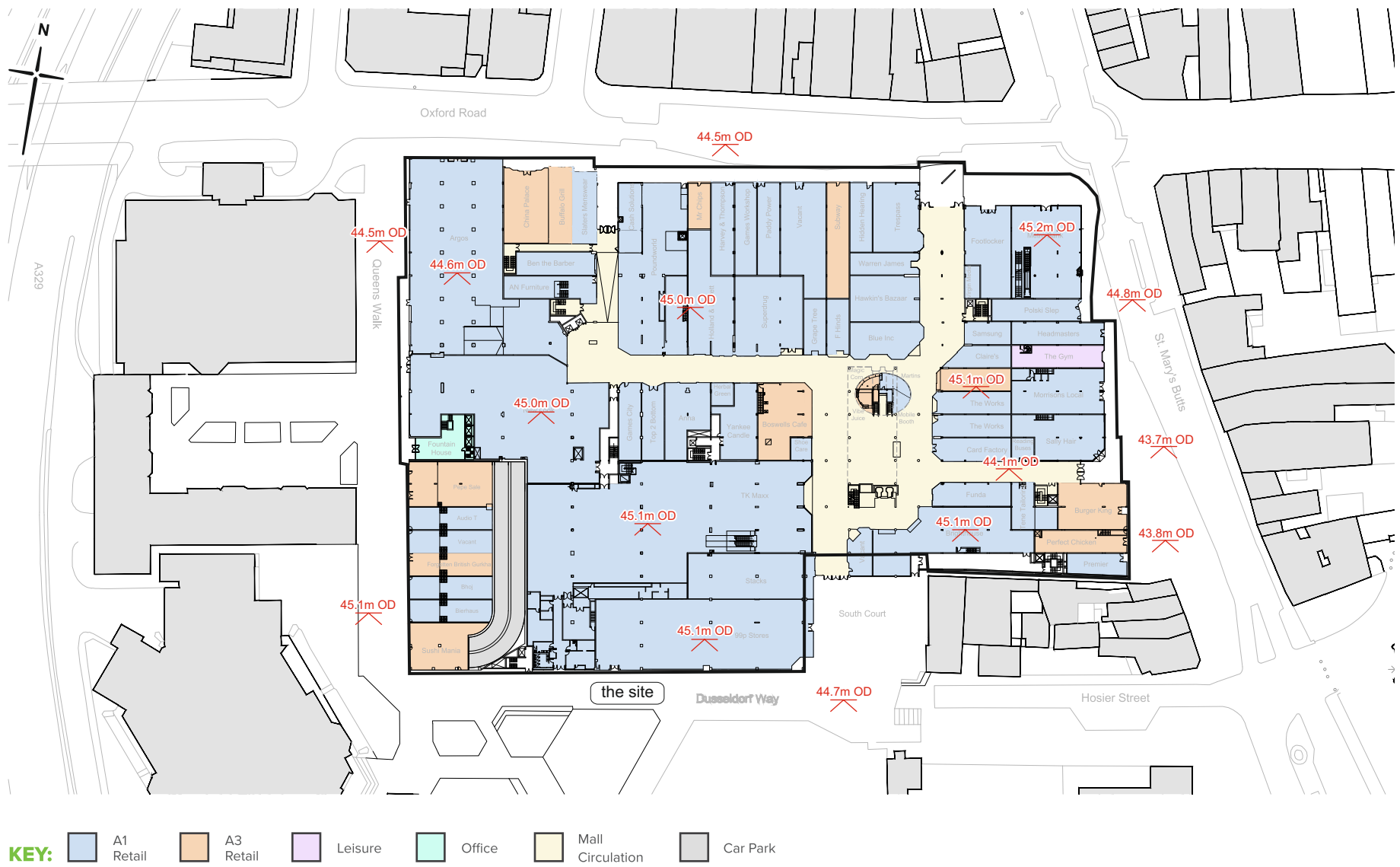
Fig 4a Existing ground floor plan showing levels taken from site survey (Corstorphine and Wright Architects, October 2016; Warner Surveys, Job No.S715/0357, May 2017)
