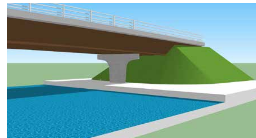
Figure 79. Retaining wall with column and embankment
