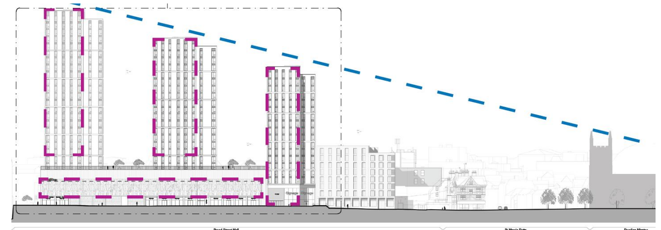
Figure 3.5 Down grading of Buildings A to C
