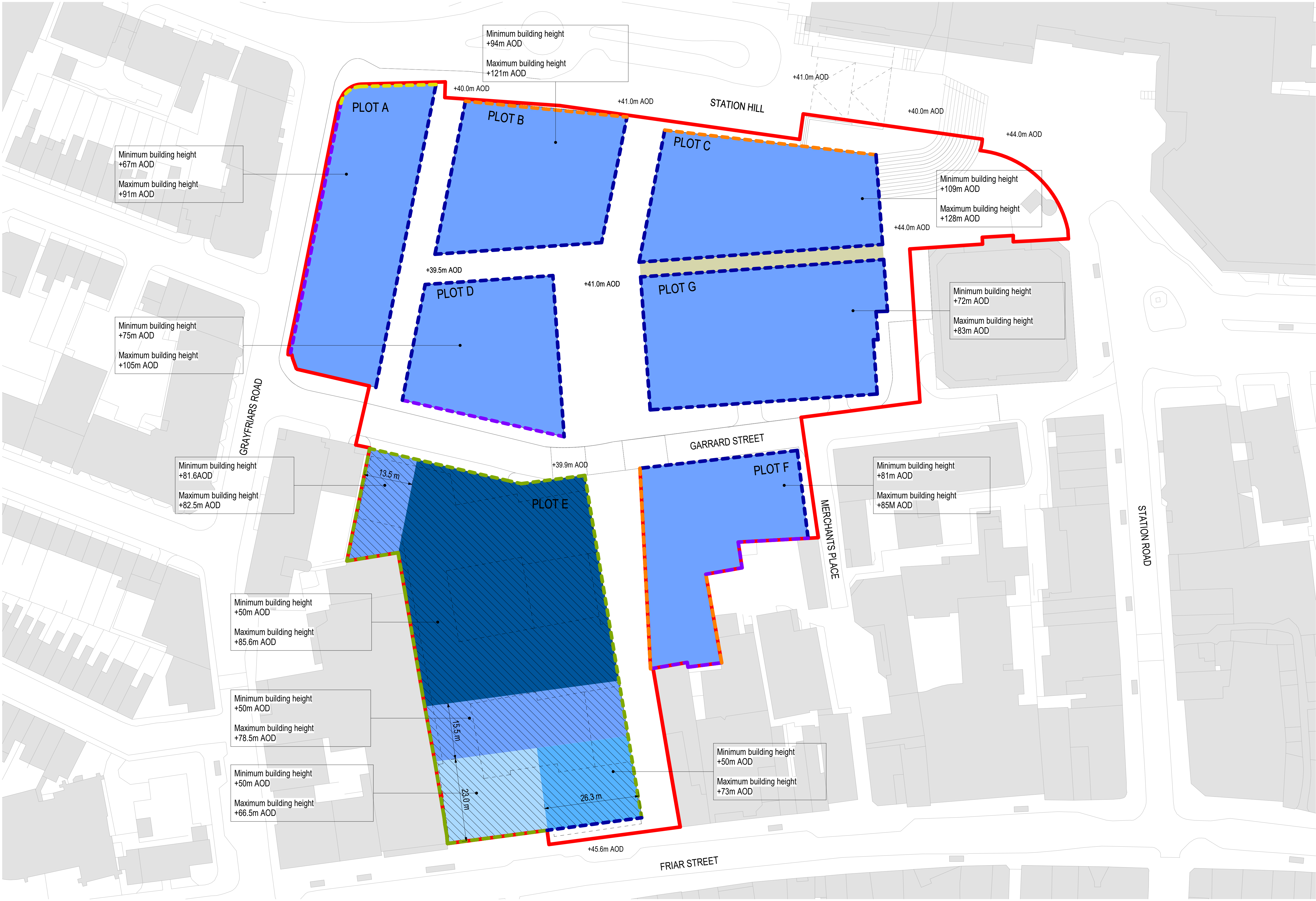
Parameter Plan_Block E - Building Plots
