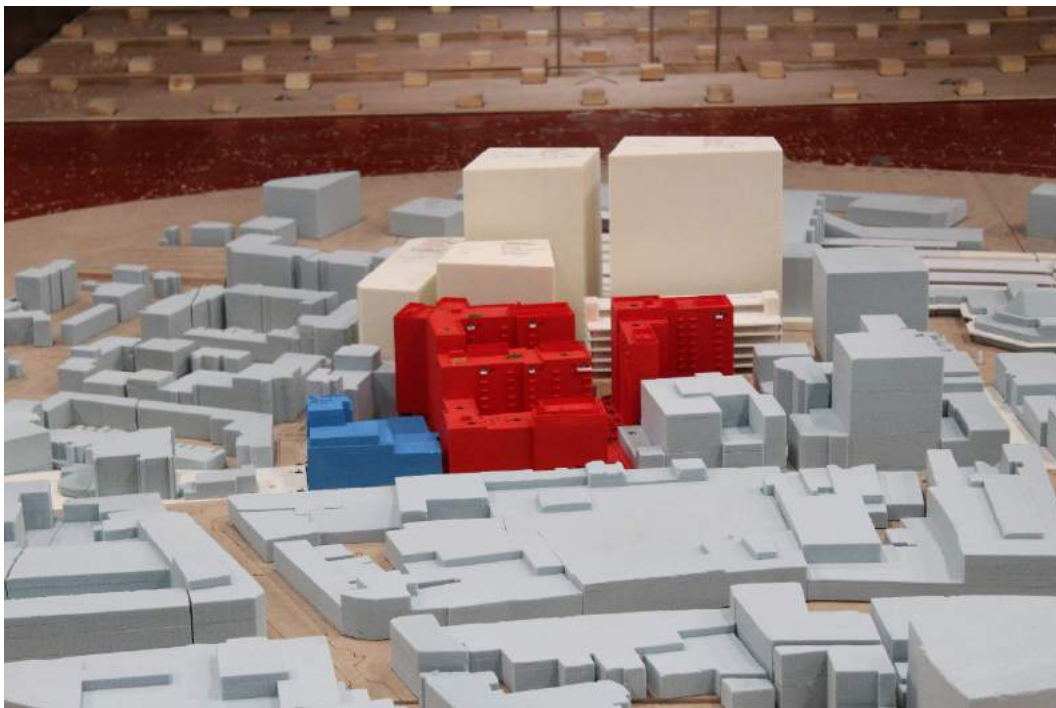
Figure 19: Proposed Development with Mitigation comprising reserved matters details for Plots E and F with the remaining Station Hill Development (as maximum parameters) in place and wind mitigation measures (Configuration 3) – View in the Wind Tunnel (from the south)
