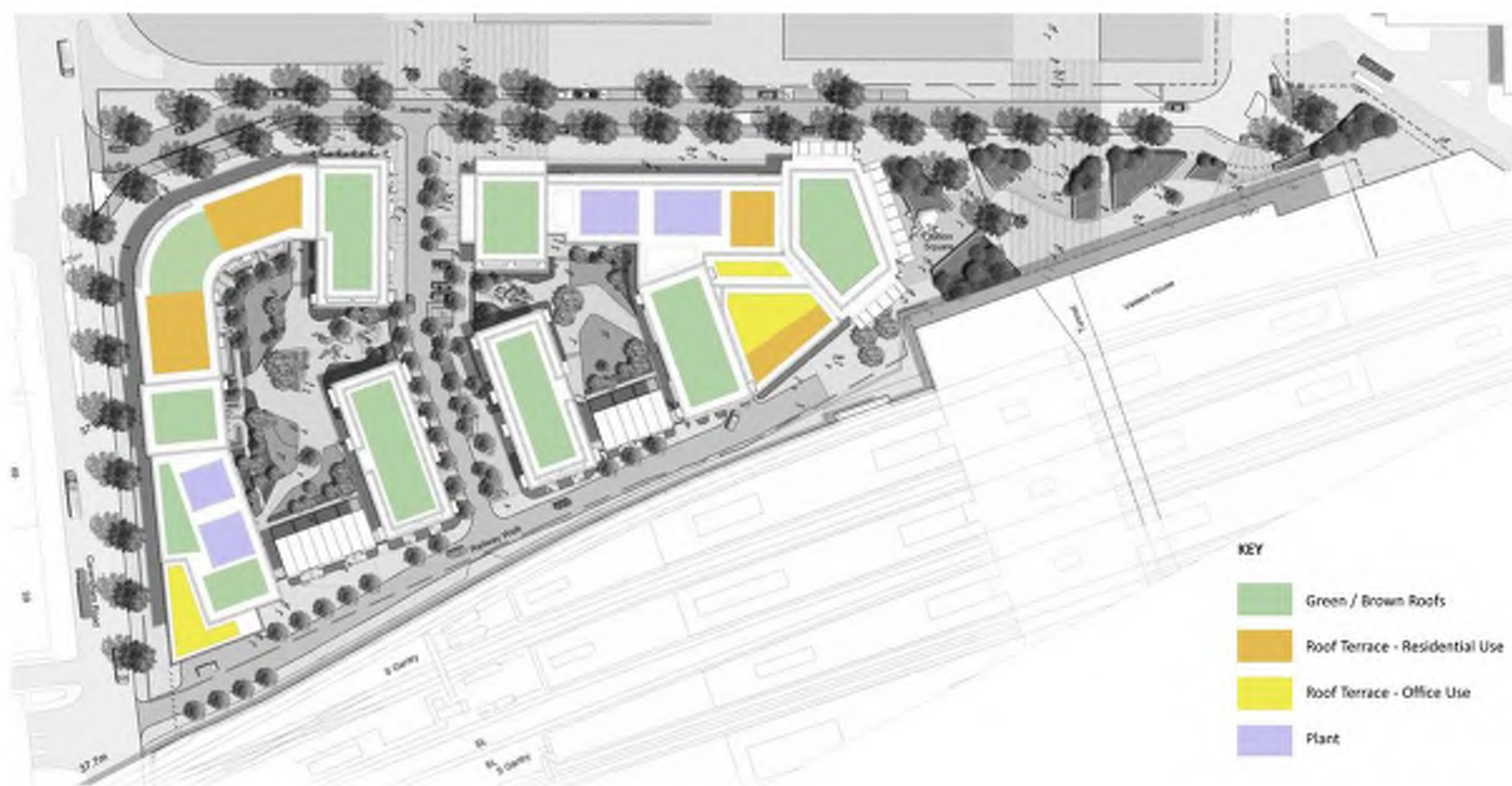
Figure 39. Roofspace Location & Types
