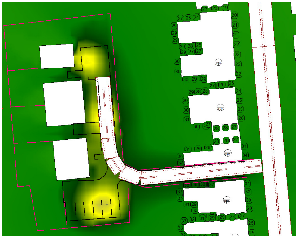
Figure 5: Night-time L_{Aeq1hour} noise levels predicted at 29 and 31 Blenheim Road
