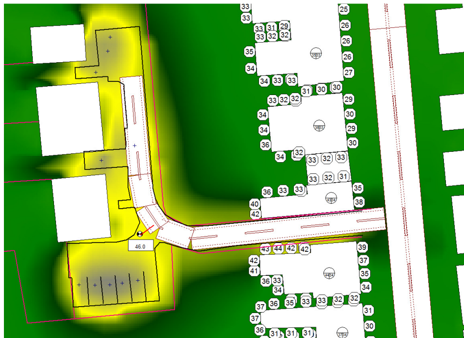
Figure 5: Night-time L_{Aeq1hour} noise levels predicted at 29 and 31 Blenheim Road
