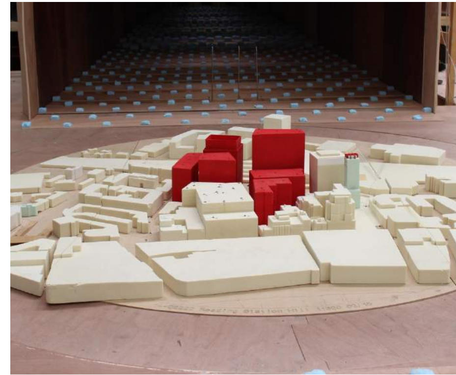
Figure 17: Completed Development (maximum parameter massing) with cumulative surrounds (Configuration 4) – View in the Wind Tunnel (from the South)
