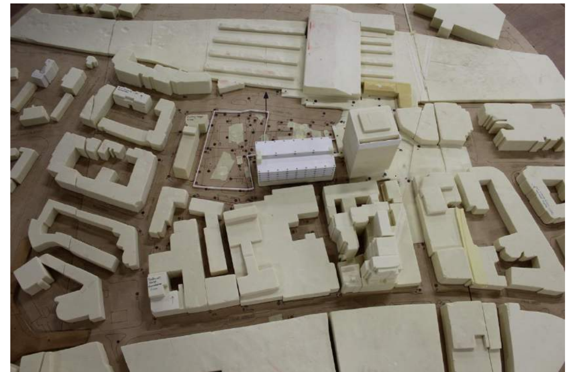
Figure 14: Temporary scenario with temporary events space (Configuration 2) – View in the Wind Tunnel (from the South, overhead)
