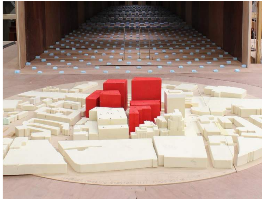
Figure 15: Completed Development (maximum parameter massing) with existing surrounds (Configuration 3) – View in the Wind Tunnel (from the South)
