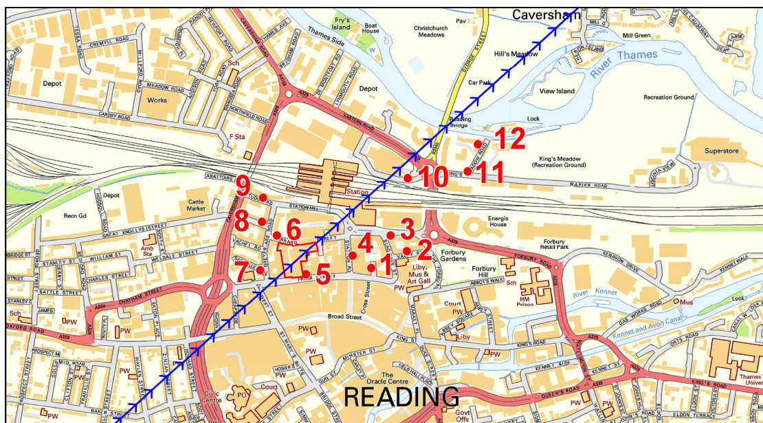
Figure 9 - Surveyed Locations. The blue arrows indicate the direction of the incoming DTT signals from the Hannington transmitter
