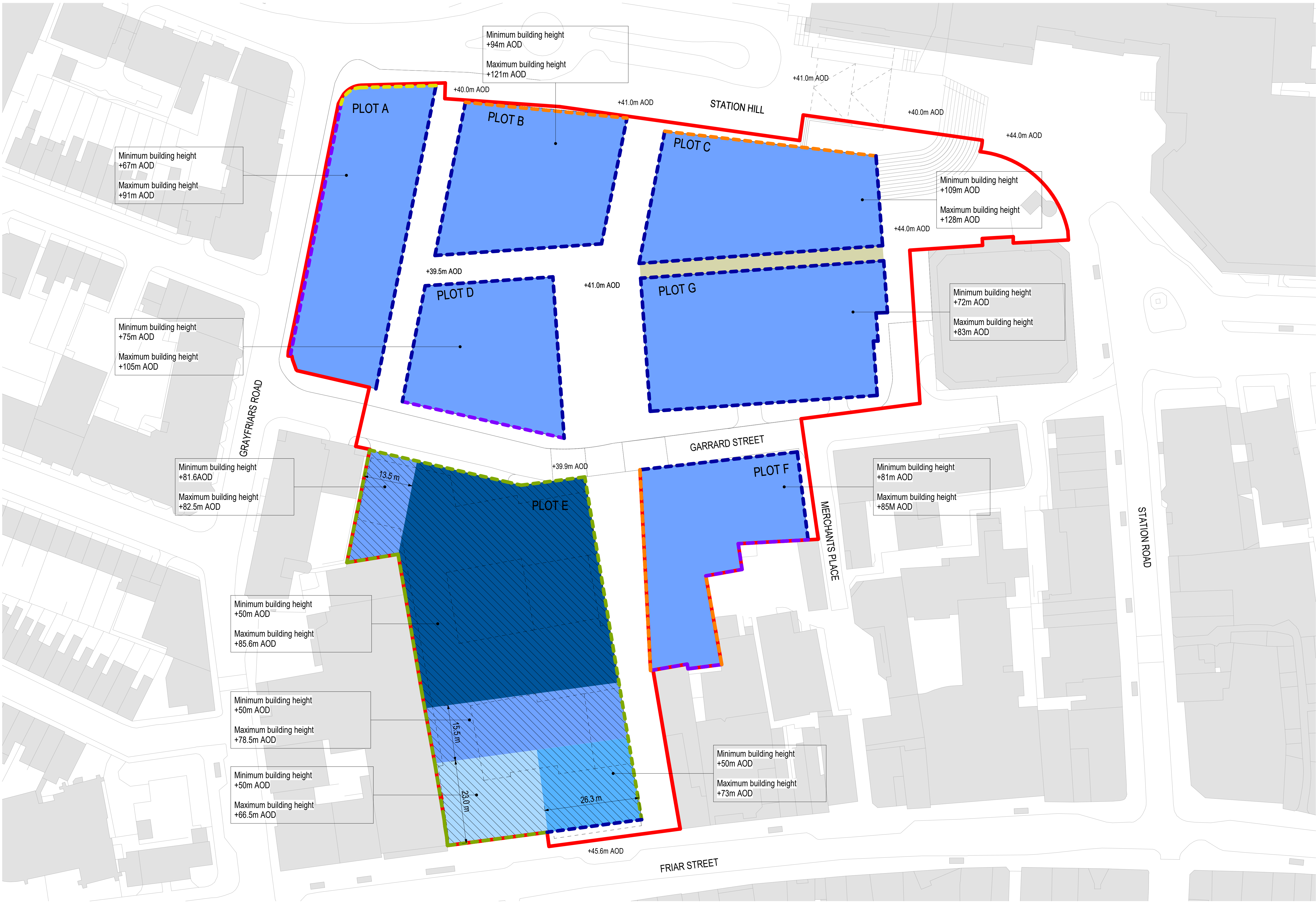
Parameter Plan_Block E - Building Plots
