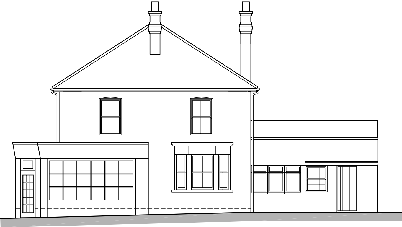
Existing Side Elevation Scale 1-100
