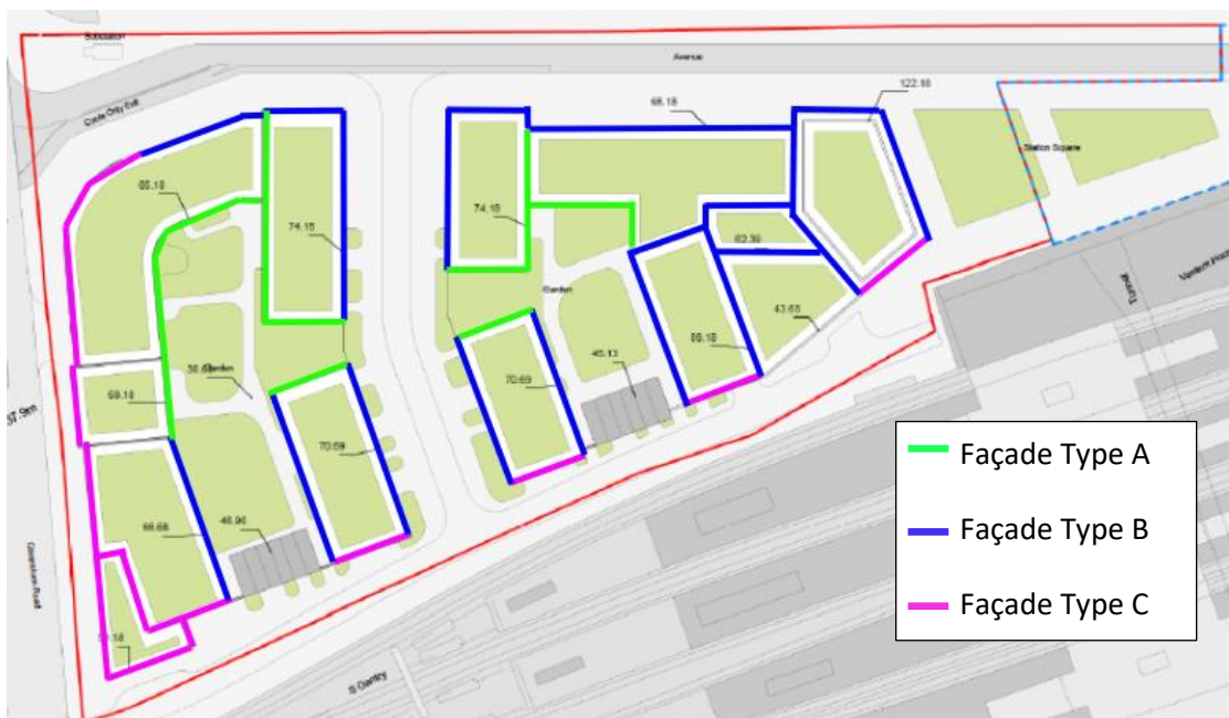
Figure 4: Façade Noise Levels
