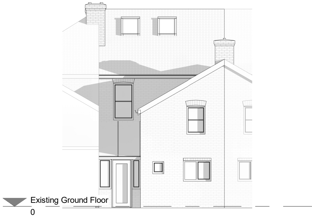
Existing Rear Elevation 1 : 100
