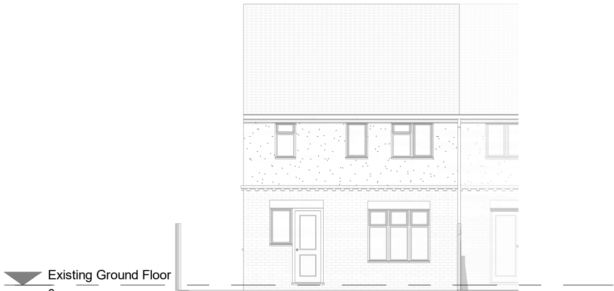
Existing Rear Elevation 1 : 100
