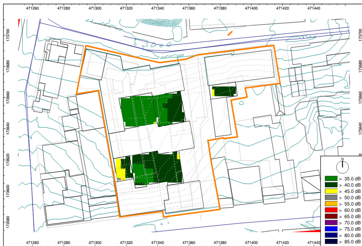
Figure 6: Predicted L_{Aeq,16hr} daytime noise level at 1.5m above each external residential terrace.
