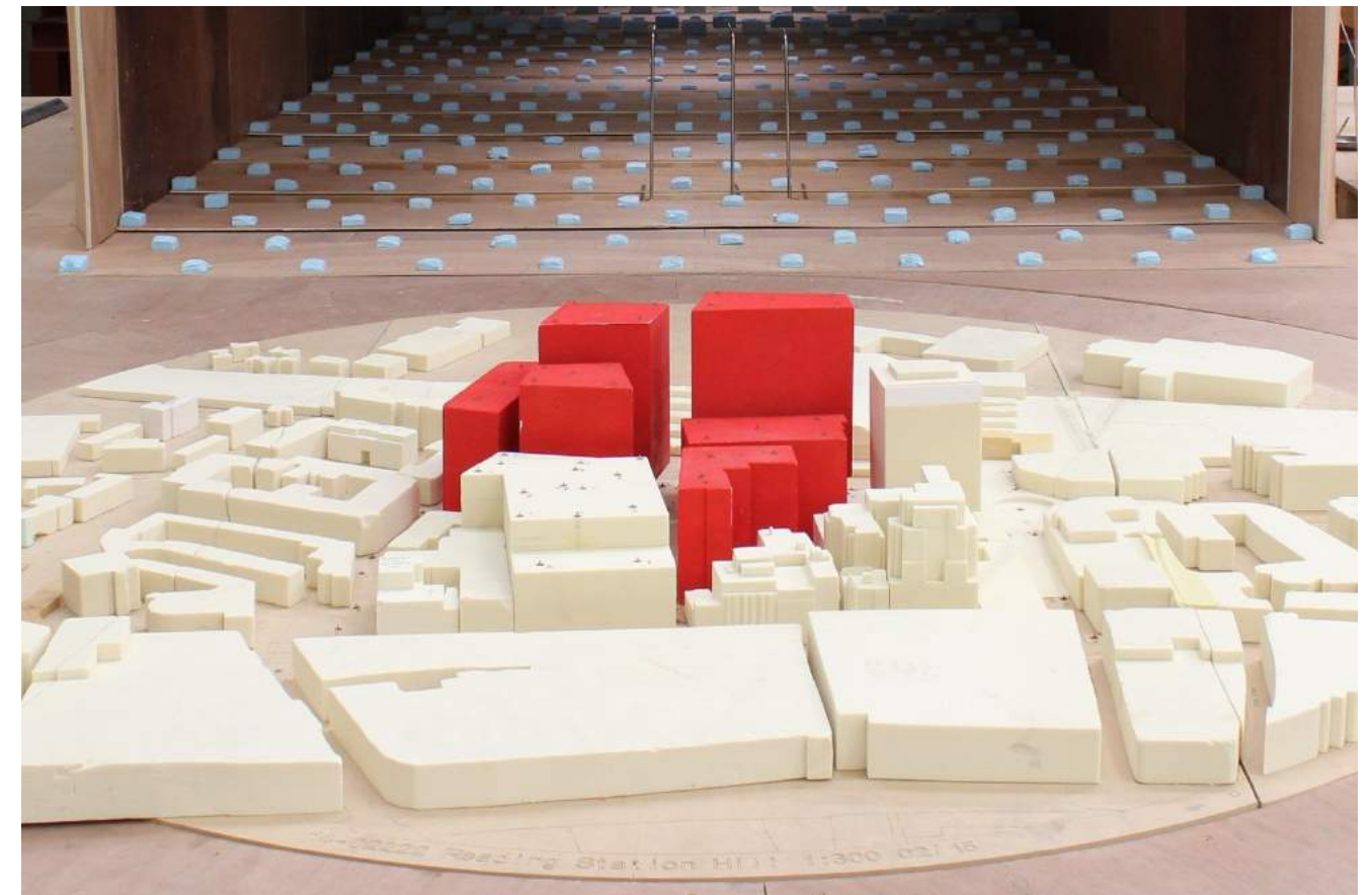
Figure 2: Image of the Proposed Development –Configuration 3 in the Wind Tunnel (view from the South)
