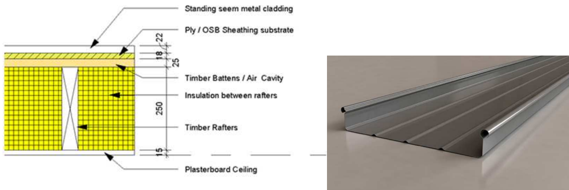
Figure 3.10: Typical standing seam roof system
