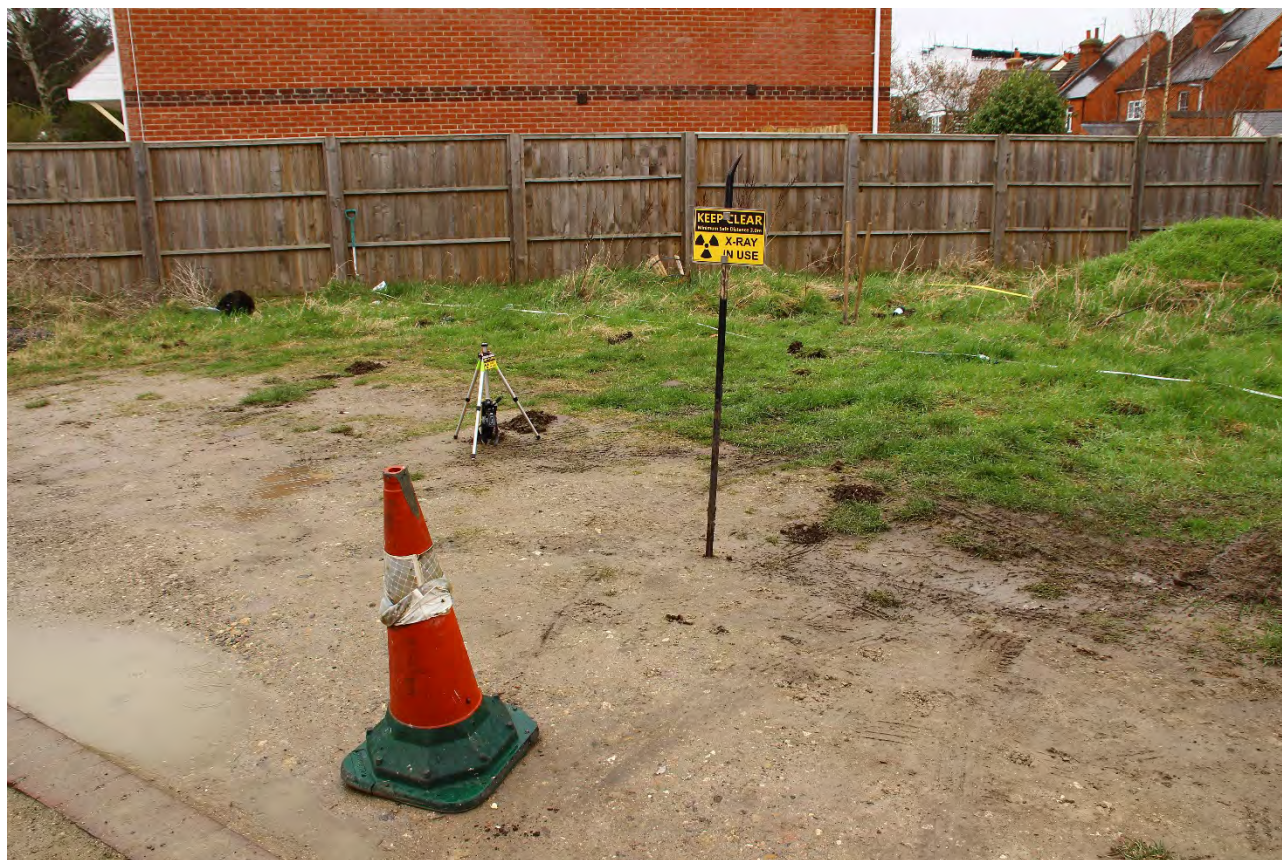
Above, the site area being tested using an XRF analyser
