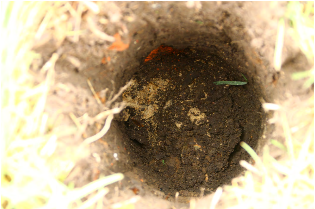
Above, a view inside HD1 showing the pale brown clayey sand below the topsoil/made ground
