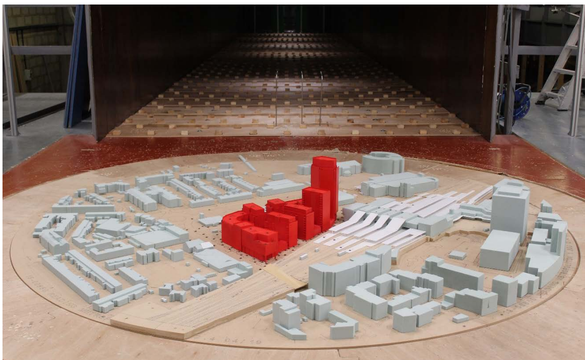
Figure 2: Image of the Proposed Development with Existing Surrounds in the wind tunnel (view from the south-west).
