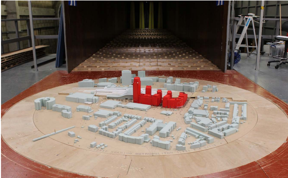
Figure 15: Mitigation: Proposed Development with landscaping, mitigation and existing surrounding building – View in the Wind Tunnel (from the North).
