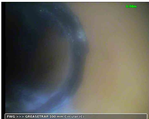
20190529-155231-snap0002.jpg, 00:00:40, 0.08 m Survey abandoned, WOULD NOT TRAVERSE AROUND CORNER
