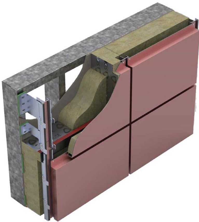
Example wall buildup
