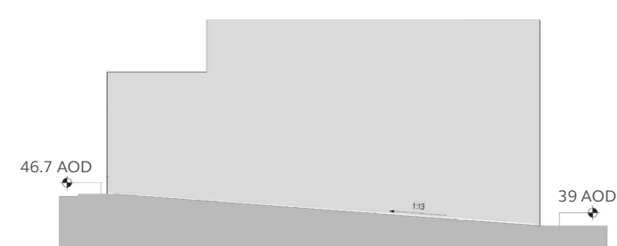
Section through the illustrative proposal for Friars Walk showing changes in level from Friar Street to Garrard Street, a slope of 1:13 which would be difficult to use for less-able people
