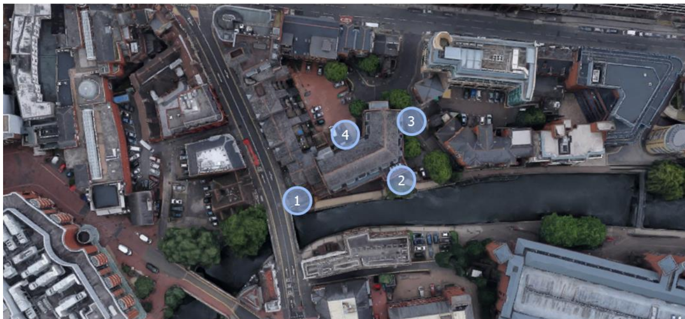
Figure 4: On Site Sound Pressure Level Measurement Positions
