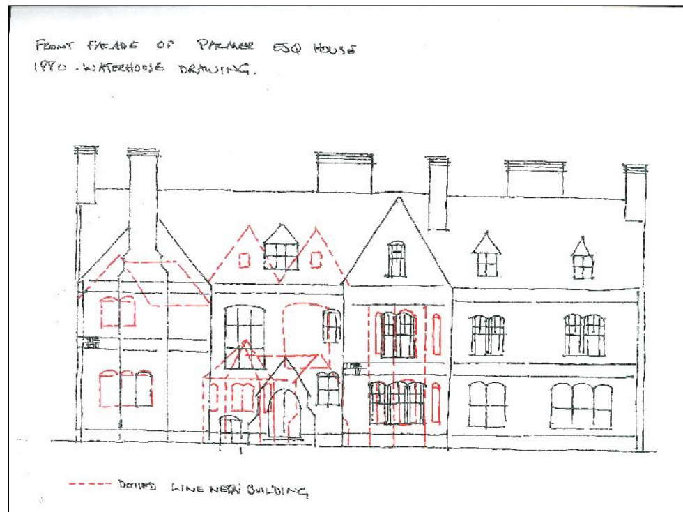
Figure 9: A plan to show the latter extensions by the University to the east elevation/front facade of East Thorpe in 1962/3 and 1973/4. 13
