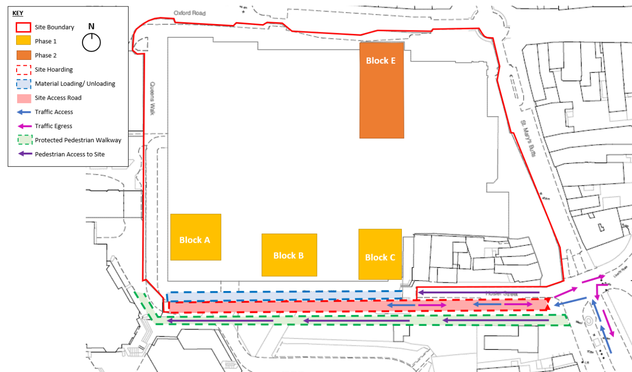
Figure 5.5 Site Establishment and Logistics Layout Plan
