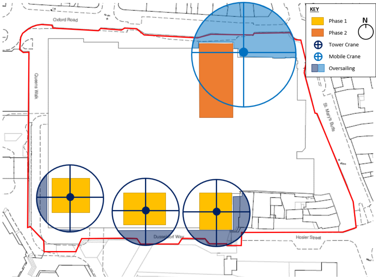
Figure 5.7 Proposed Tower Crane Location and Radius
