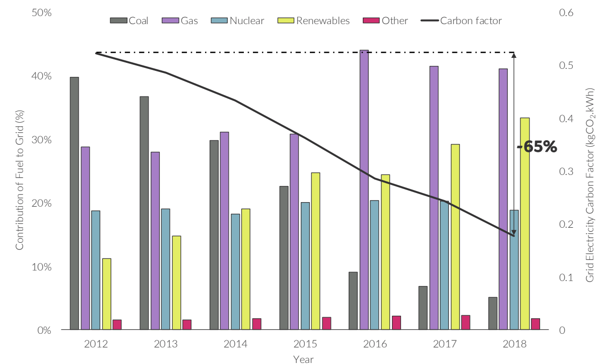
Figure 11: Historic mix of generation methods and associated carbon factor for the National Grid. Transmission and distribution losses are included. Sources: OfGem (generation mix); BEIS Green Book (historic carbon factors).
