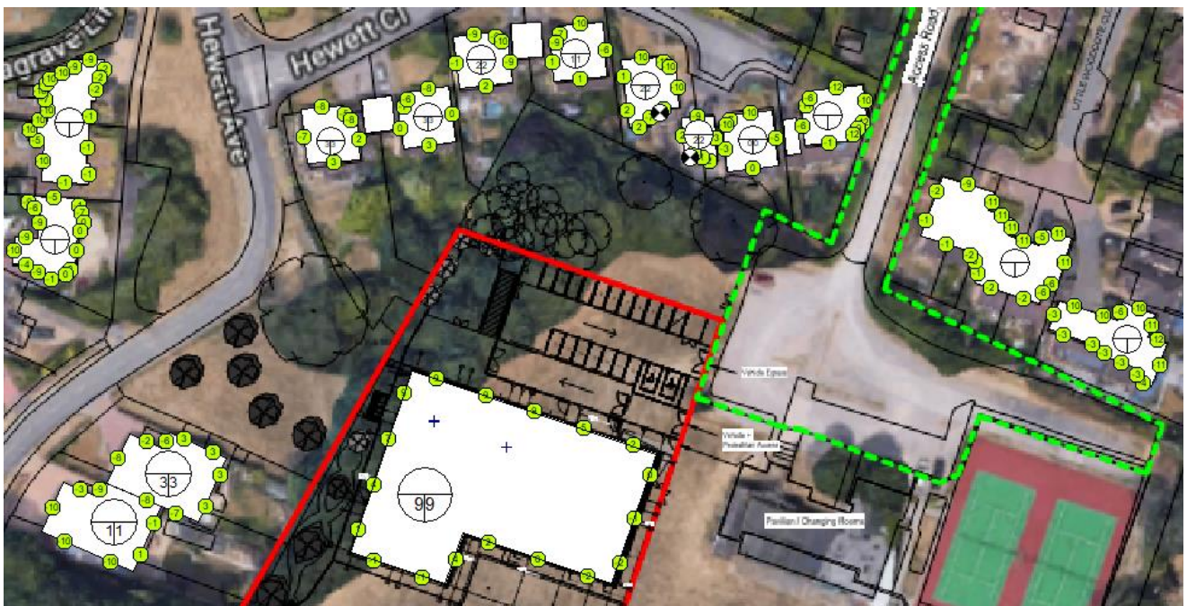
Figure 3.6: Noise Mapping of Proposed Plant Noise Breakout at night-time
