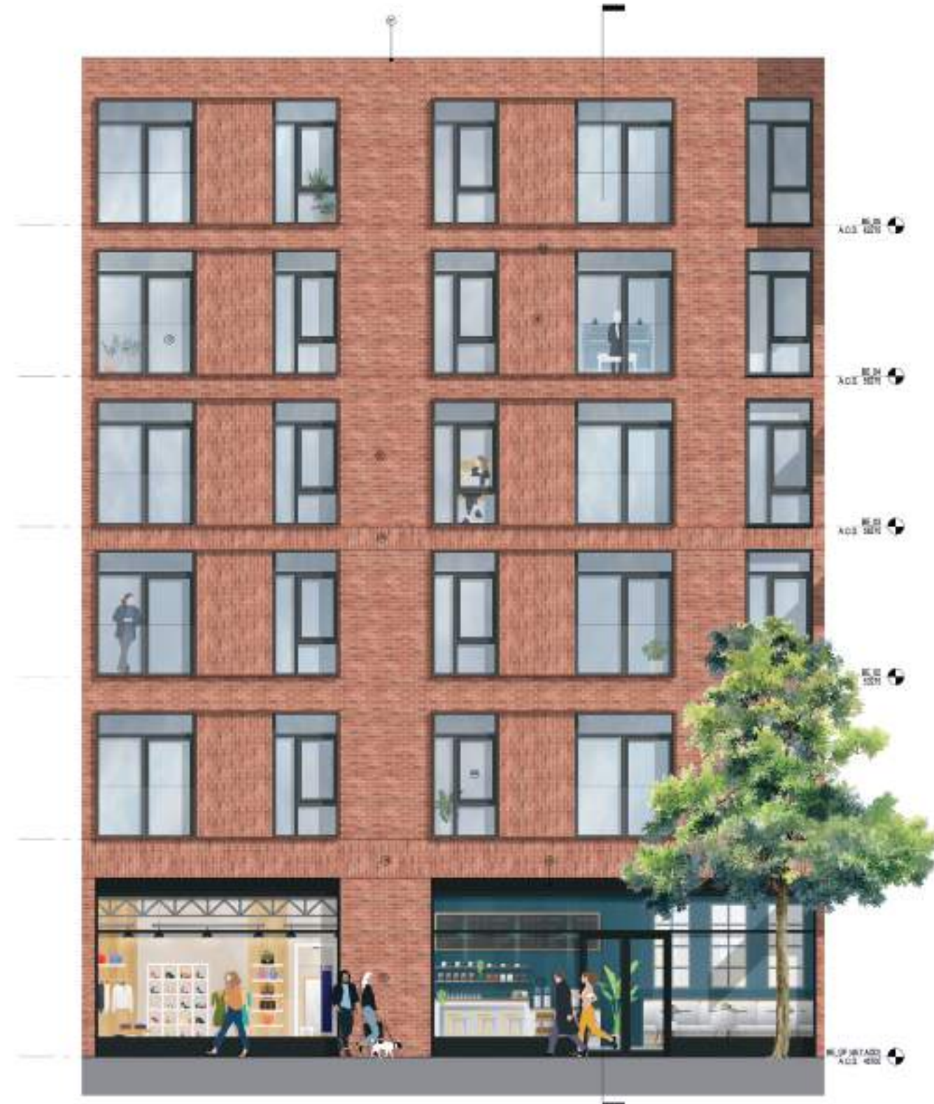
1 Plot E - Friar Street - Brick - Bay Elevation 1:30
