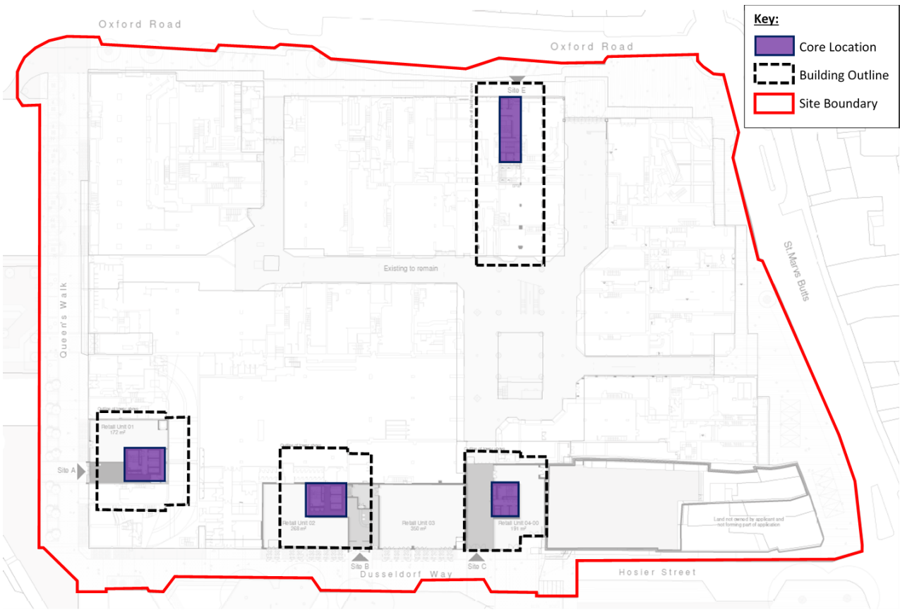
Figure 3.5 Residential Building Core Locations
